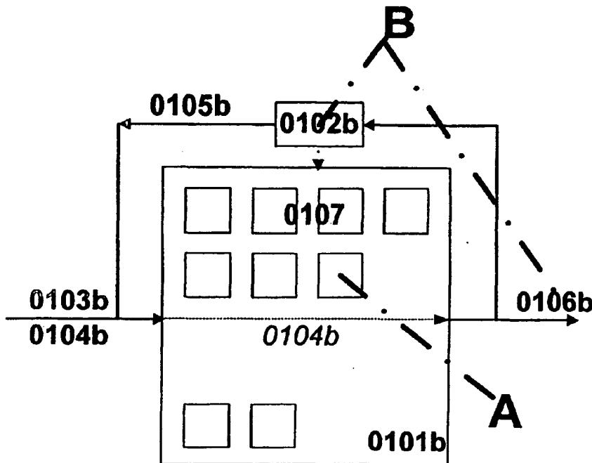
(57) Abstract: The invention relates to a method for debugging reconfigurable hardware. According to the inventive method, all necessary debug information for each configuration cycle is written into a memory which is then evaluated by the debugger.
